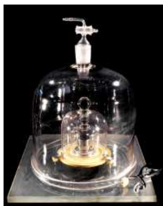
Figure 3: The International Prototype of the Kilogram (Reproduction Authorized, BIPM, www1.bipm.org/en/scientific/mass/prototype.html )
