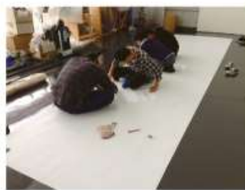
設計図を元に型紙を作成し、農業用フィルムを切断 Making a paper pattern basis on blueprint, and cutting films
