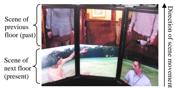
Figure 3: Scene movement giving a feeling as if elevator goes downward
